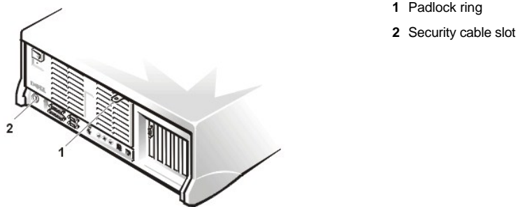
Figure 4. Mini Tower Chassis Security Cable Slot and Padlock Ring
